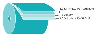
This flexible packaging material is designed for both stand-up pouch formats and form, fill and seal processes. In addition to being ideal for wet and dry goods, this structure provides superior scratch resistance, toughness and is surface imprintable, while offering superior moisture and oxygen barriers.
