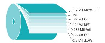
This flexible packaging material is designed primarily for form, fill and seal processes. This structure is used for packaging of dry, wet and liquid goods. It is heat sealable and the foil core provides superior moisture, oxygen and light barriers. This structure provides superior scratch resistance, toughness and is surface imprintable.
