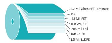
This flexible packaging material is designed primarily for form, fill and seal processes. This structure is used for packaging of dry, wet and liquid goods. It is heat sealable and the foil core provides superior moisture, oxygen and light barriers. This structure provides superior scratch resistance, toughness and is surface imprintable.
