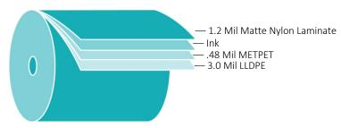
This flexible packaging material is designed for both stand-up pouch formats and form, fill and seal processes. In addition to being ideal for wet and dry goods, this structure provides superior scratch resistance, toughness and is surface imprintable, while offering superior moisture and oxygen barriers. The nylon component of this material offers superior puncture resistance integrity to the film.
