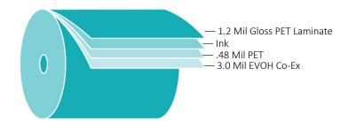
This flexible packaging material is designed for both stand-up pouch formats and form, fill and seal processes. In addition to being ideal for wet and dry goods, this structure provides superior scratch resistance, toughness and is surface imprintable, while offering superior moisture and oxygen barriers.
